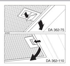
To remove the grease filters release the latch. Holding carefully, lower and remove the filter.
